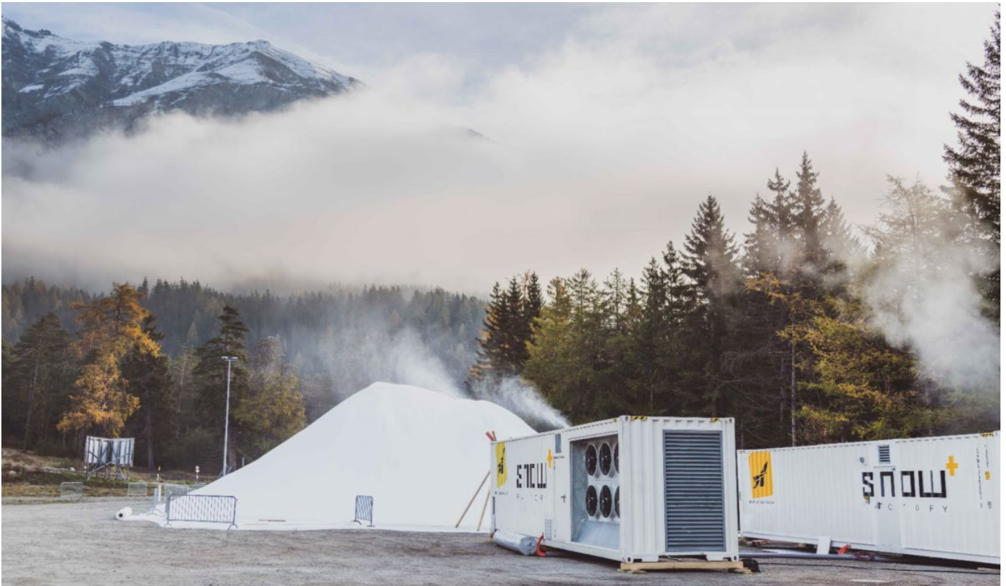
The Snow Factory (above) is capable of producing snow at temperatures above 60 degrees. Photo: Courtesy of TechnoAlpin
